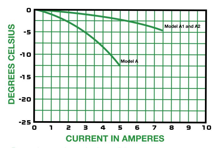
These are only representative curves based on controlled laboratory testing. Results may vary in actual applications.
