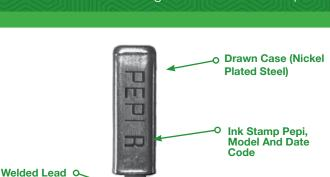
**Model R** units are normally in the closed position allowing electricity to flow through the circuit. When the temperature exceeds a preset high limit, the bimetal element open to break the circuit. When the temperature cools, the bimetallic element returns to its original shape closing the circuit.
