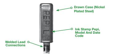
**Model L** units are normally in the closed position allowing electricity to flow through the circuit. When the temperature exceeds a preset high limit, the bimetal element open to break the circuit. When the temperature cools, the bimetallic element returns to its original shape closing the circuit.
