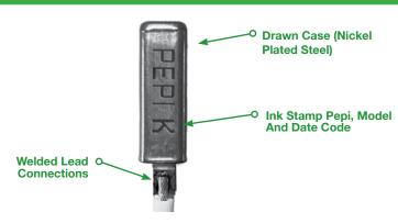
Model K and -K units are normally in the closed position allowing electricity to flow through the circuit. When the temperature exceeds a preset high limit, the bimetal element open to break the circuit. When the temperature cools, the bimetallic element returns to its original shape closing the circuit.
