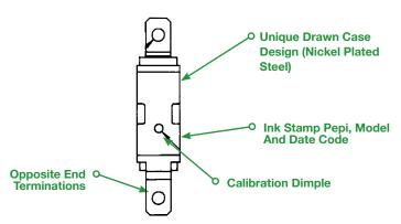
Model E units are normally in the closed position allowing electricity to flow through the circuit. When the temperature exceeds a preset high limit, the bimetal element open to break the circuit. As temperatures cool, the bimetal element eases back to its original shape, closing the circuit.
